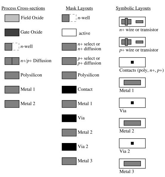
Diffusion areas are where n+, p+ have been introduced to form source, drain, and well-contacts areas.
