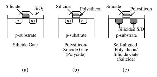
Cross-section (a): Gate is made of a <u>silicide</u>—polysilicon combined with tantalum (other metals can be used). Sheet resistance  $\Rightarrow 1$  to 5 $\Omega$  per square
