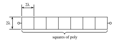
7 squares; if  $30\Omega/\text{sq}$ . then  $R_{\text{end-to-end}} = 30 \times 7 = 210\Omega$ .
